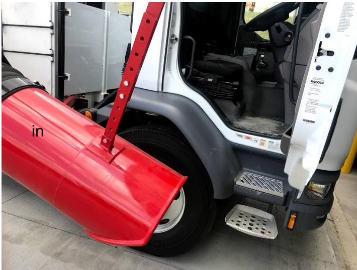
Easy operator entrance when hose is in locked travel position
