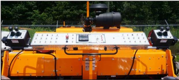
**Propulsion Controls:** Dual electronic joystick controls provide forward and reverse direction with steering from either side of the paver.
