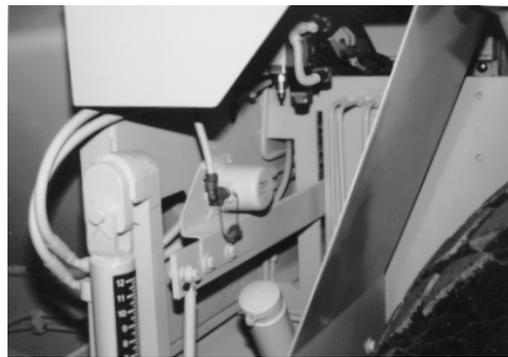
Slope Sensor, 400 and 500 Series Pavers
