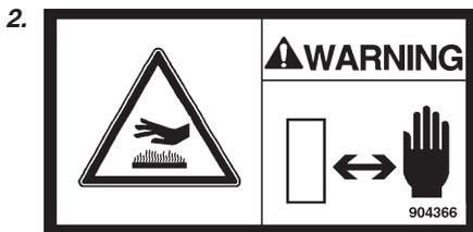
Warning - hot surfaces in the engine compartment. Do not touch.
