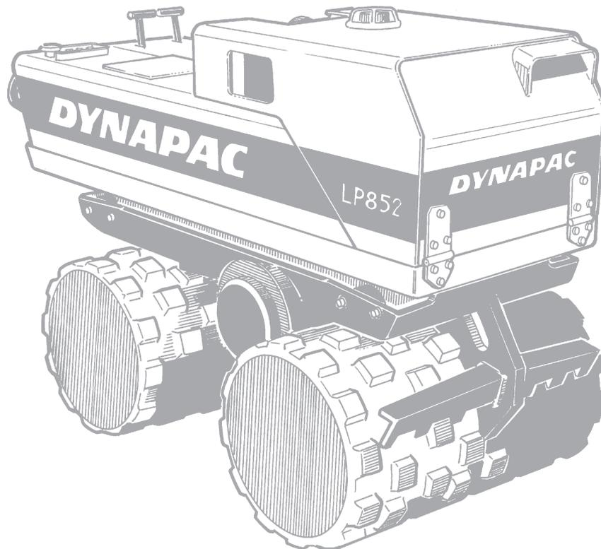
*Dynapac LP 852 is a vibratory padfoot roller that is designed to cope with many different types of compaction work. The roller is designed essentially for compaction tasks in pipe trenches, around the foundations of buildings, backfilling against supporting walls, and also for road construction. The machine is equally suitable for work in confined spaces as for major compaction jobs.*
