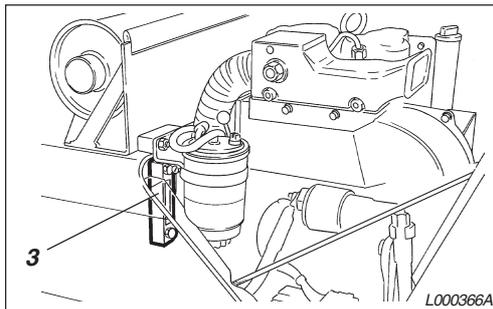
1. Wipe of the oil level gauge (3) and check that the level is in the middle of the glass. If necessary fill up (4). If the level is sinking check for leakage.
