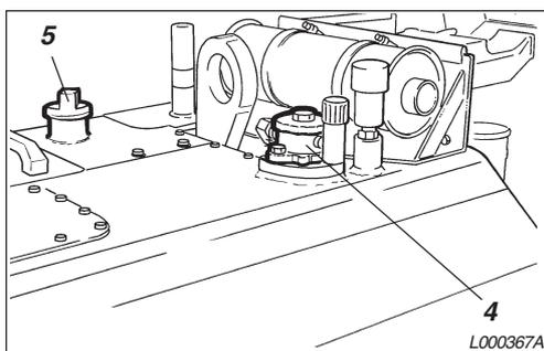
1. Fill up fuel tank (5) every day use diesel with the following specifications.
