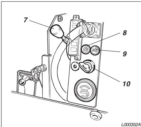
10. Adjust the speed control (7) and let the engine idle for 5 - 10 minutes depending on air temperature.
