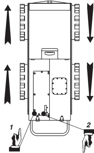
Turning the machine to the right
