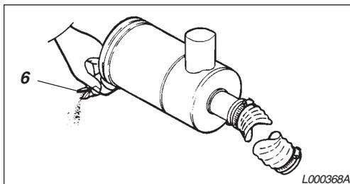
1. Check air inlet opening clean if necessary
