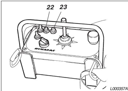
8. Turn the starter key (10) (or press down on/off-button (22) IR-control) which activates the main-relay, check that lamps for charge (8) and oil pressure (9) lights up. Open cover (29) and check.
