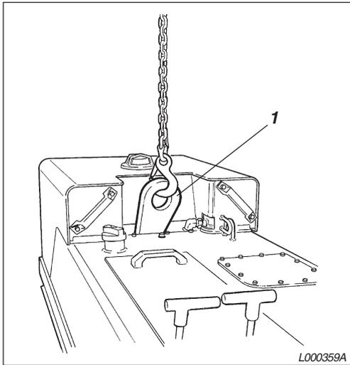
**Machine ready for lifting**
