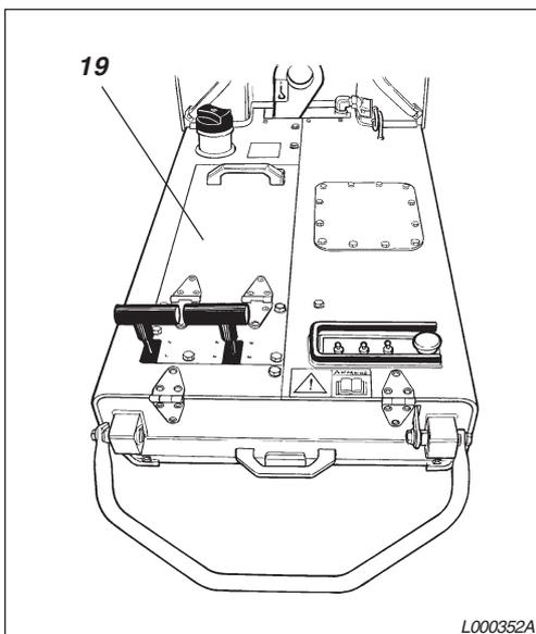
The IR transmitter (19) and the receiver unit, including the charging cable, are located under the cover; see under the "Controls-Cable and IR control" heading.
