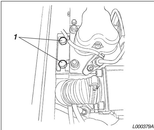
Ensure that the engine spacer bolts are properly tightened.
