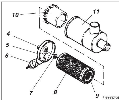
1. Undo wing nut (4) and remove cover (5) with dust-extractor valve (6).
