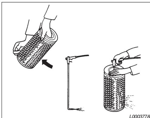
1. Tap the filter cartridge against the ball of your hand until no more dust falls out. Do not knock the filter cartridge against hard objects.
