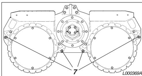
1. Make sure that every scraper do not touch the pads on the drums. Adjust if necessary distance to 3-5 mm (0.1-0.2 in). With screws (7).
