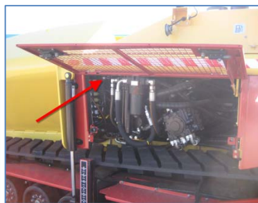
Fig.2 Connecting hydraulic accumulator and nitrogen bottle
