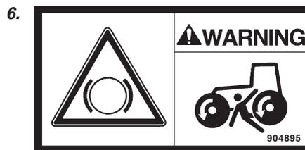
Study the towing chapter before disengaging the brakes. Danger of being crushed.
