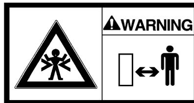
Crush zone, articulated steering. Maintain a safe distance from the crush zone.
