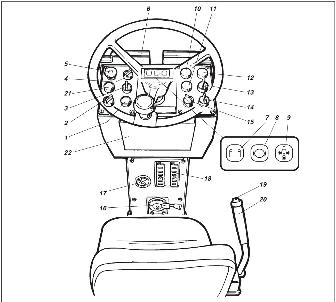
**Fig. 6 Instruments and control panel**
