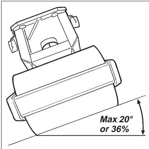
Fig. 2 Tipping angle on side slopes
