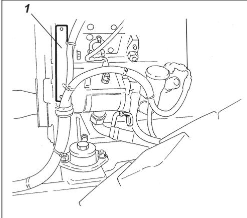
The engine data plate (1) is affixed to the right side of the engine under the injection pump. The plate indicates the type of engine, serial number and engine data. Please state the engine serial number when ordering spare parts. See also the engine manual.
