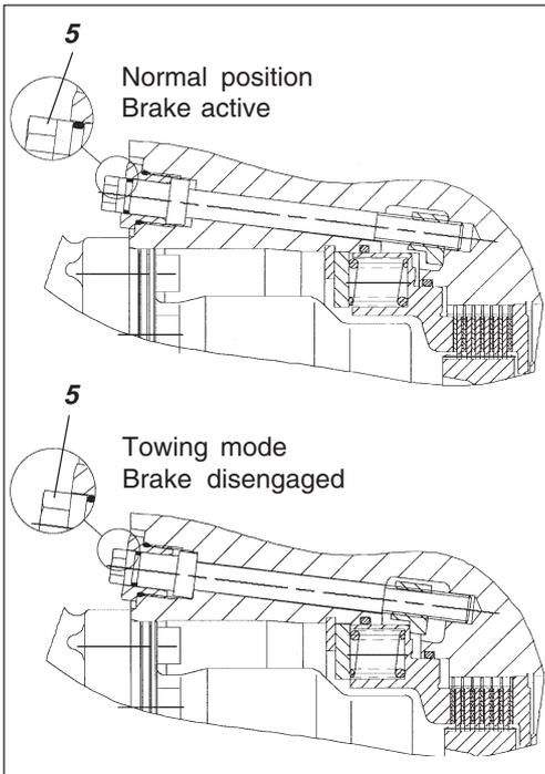
**Fig. 29 Drum brake**
