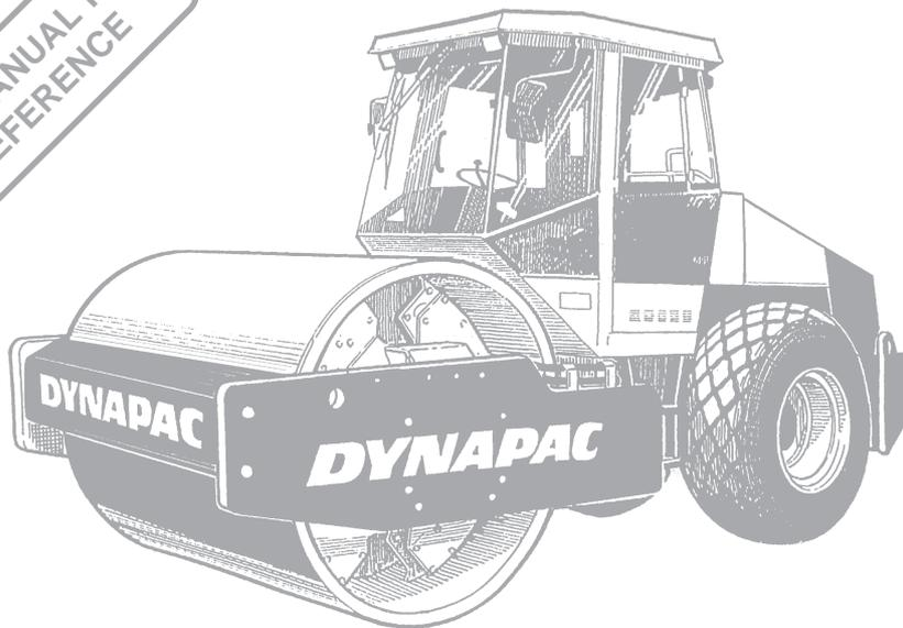
*The Dynapac CA600 is available in D (smooth drum) and PD (padfoot) versions, of which the CA600D is designed for compacting rock fill. The main range of application for the PD versions is on cohesive material and weathered stone material.*
