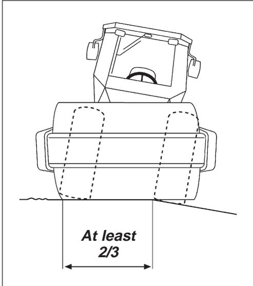
Fig. 1 Position of drum when driving near an edge
