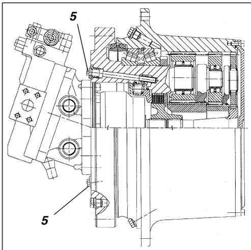
**Fig. 28 Drum brake**
