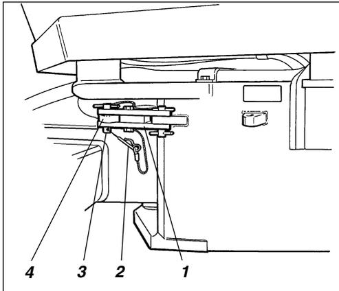
**Fig. 23** Articulation in interlocked mode
