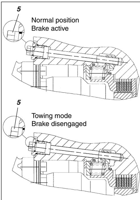
**Fig. 29 Drum brake**
