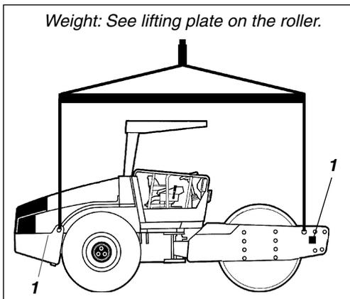
**Fig. 24** Roller prepared for lifting
