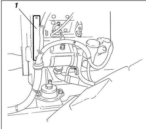
The engine data plate (1) is affixed to the right side of the engine under the injection pump. The plate indicates the type of engine, serial number and engine data. Please state the engine serial number when ordering spare parts. See also the engine manual.
